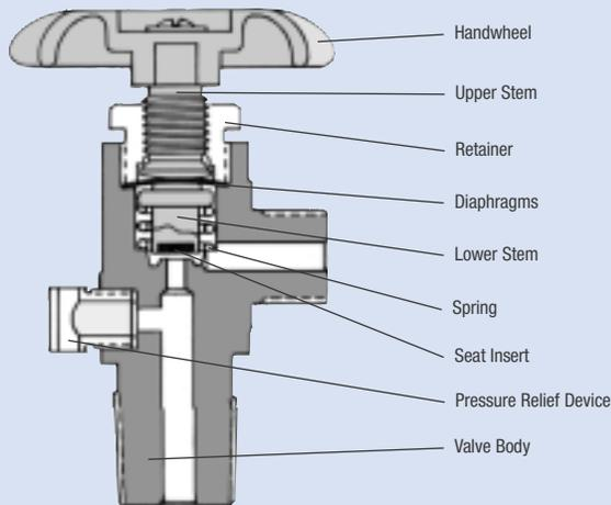
**Fig. 5****Spring-Loaded Diaphragm Valve
