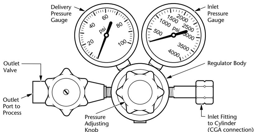
FIGURE 1, Front View – Typical Cylinder Pressure Regulator
